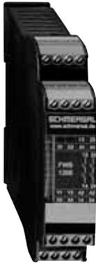
*Fig. 3: The shut-down monitors from the AZR 31 S1 and FWS ranges serve to safely record the machine shut-down. Depending on the external circuit in conjunction with a safety monitoring module from the AES or SRB range, it is possible to safeguard a protective device up to a PL “d”.*
